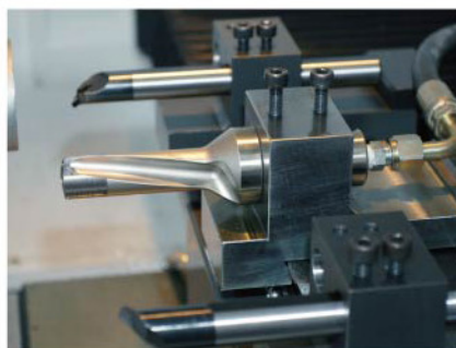
The coolant through drill option cuts the good finish holes.
