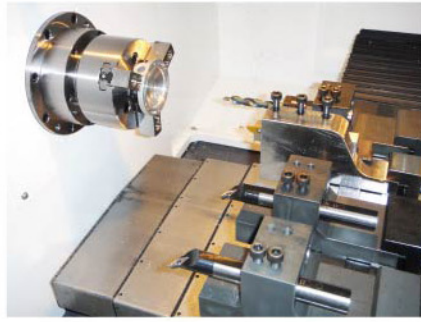
The Jaw chuck with gantry turret: The jaw chuck of 5" and 6" optional give the cutting range more flexible.
